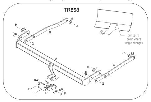
Note: 1. Recommended Torque Setting for M12 Grade 10.9 -139 Nm. (For other Torque Settings see notes overleaf.)
