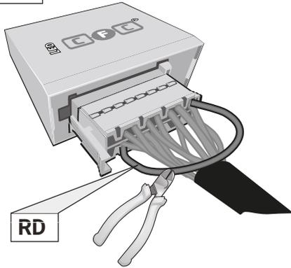
Pin 11 and Pin 2 disconnected
