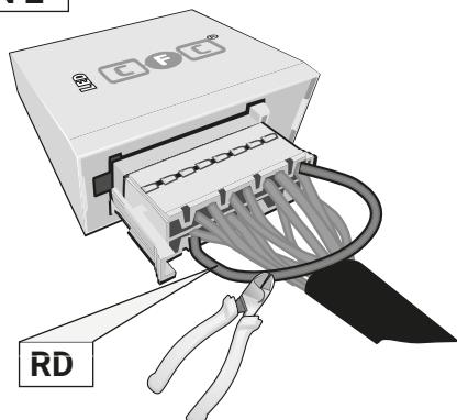
Pin 11 and Pin 2 disconnected
