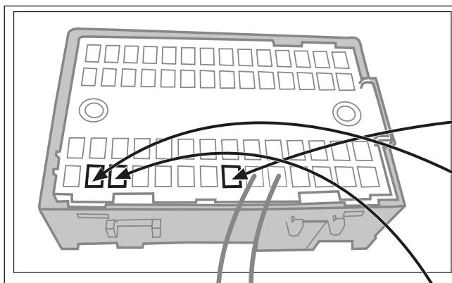
**OR RD** → Connect OR and RD into the fuse chamber 8!
