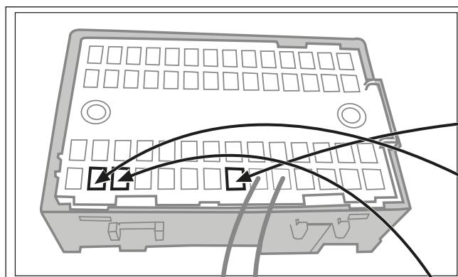
**OR RD** → Connect OR and RD into the fuse chamber 8!
