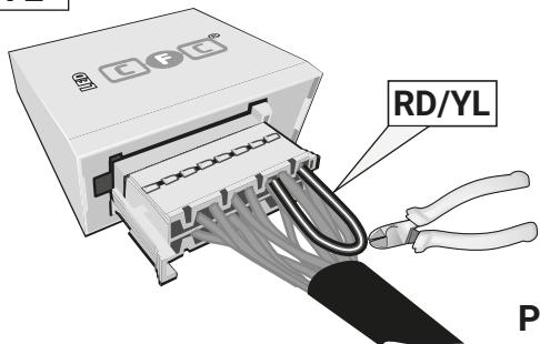
**Pin 3 and Pin 2 disconnected**
