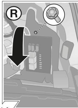
Locate 4 unoccupied fuse plug-in positions (B+/30)!
