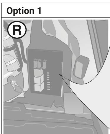
Locate 4 unoccupied fuse plug-in positions (B+/30)!
