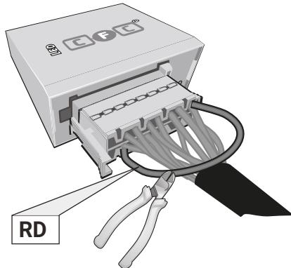
Pin 11 and Pin 2 disconnected
