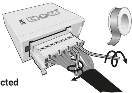
Pin 3 and Pin 2 disconnected
