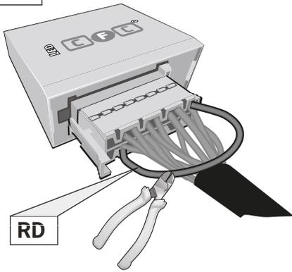
Pin 11 and Pin 2 disconnected
