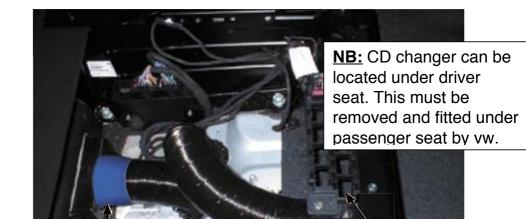
Blue silicone adapter to connect hot air outlet ducting to outlet.
