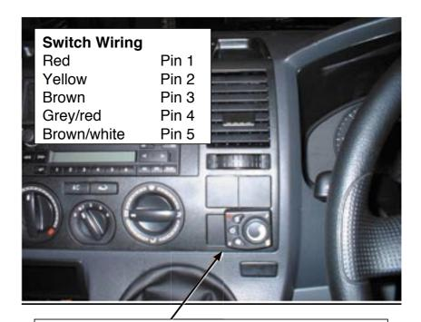
Switch mounted on dashboard onto VW blanks.
