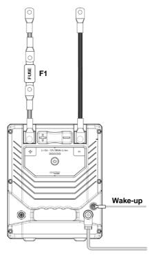
The battery has a power button to control power transfer. Activation of the battery can also be achieved through the terminal wake-up signal. The shown fuse (F1) and cable gauge should be selected according to application.
