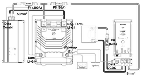
Wire the communications / control signals according to following table:
