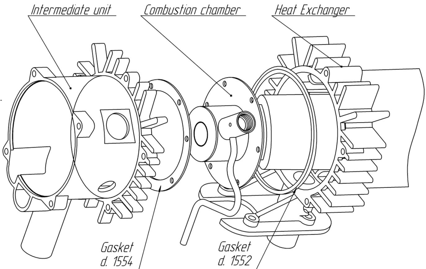
Fig.13-Combustion Camera in PLANAR-44D.
