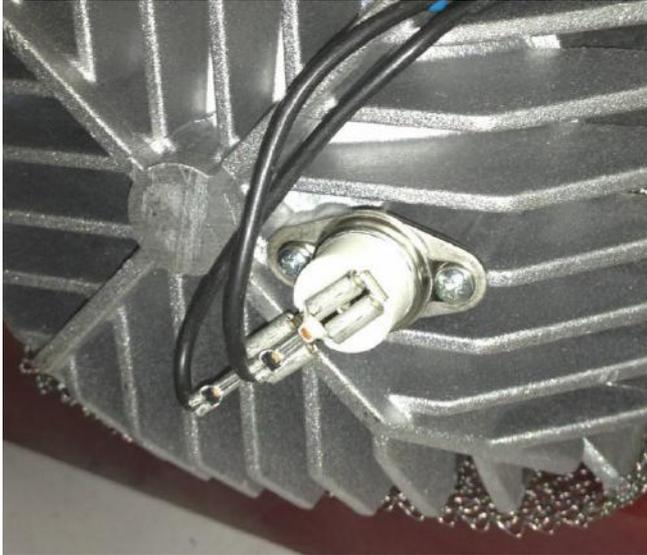
Fig.7 - Overheat sensor
