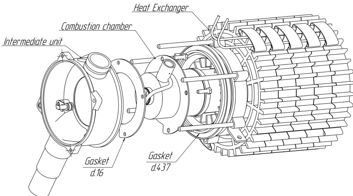
Fig.15-Combustion Camera in PLANAR-8DM.
