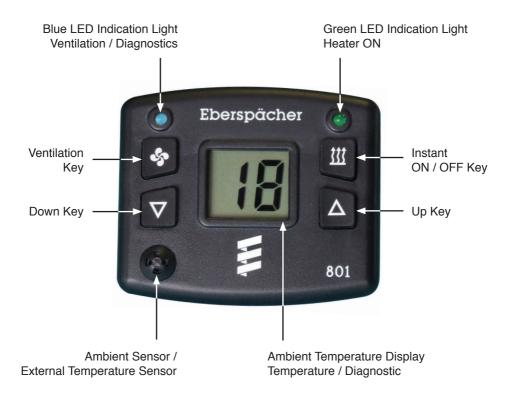
Part Number: 801 10 001 Modulator with Diagnostic Readout Instructions (1 hour run)
